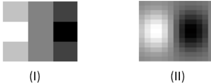
Figure 5.9: Two different types of approximations to image gradient used in experiments. (I) Sobel filter in x direction (II) Derivative of Gaussian
