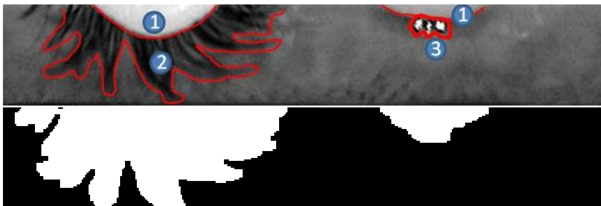
Figure 3.1: Normalized iris texture map (upper picture) and its accurate mask (lower picture), with white color indicates occluded area. In this iris map, there are noises caused by (1) eyelids, (2) eyelashes, and (3) specular reflections, as indicated in the picture. All of these artifacts have to be indicated in the mask in order to achieve high recognition performance.
