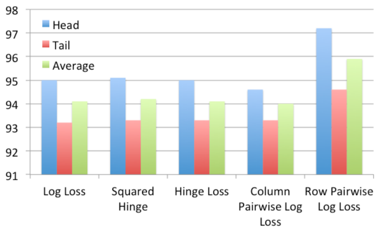
Figure 6.3: The Hits@10 scores of different loss functions for learning embeddings to retrieve head and tail entities on the WordNet dataset.
